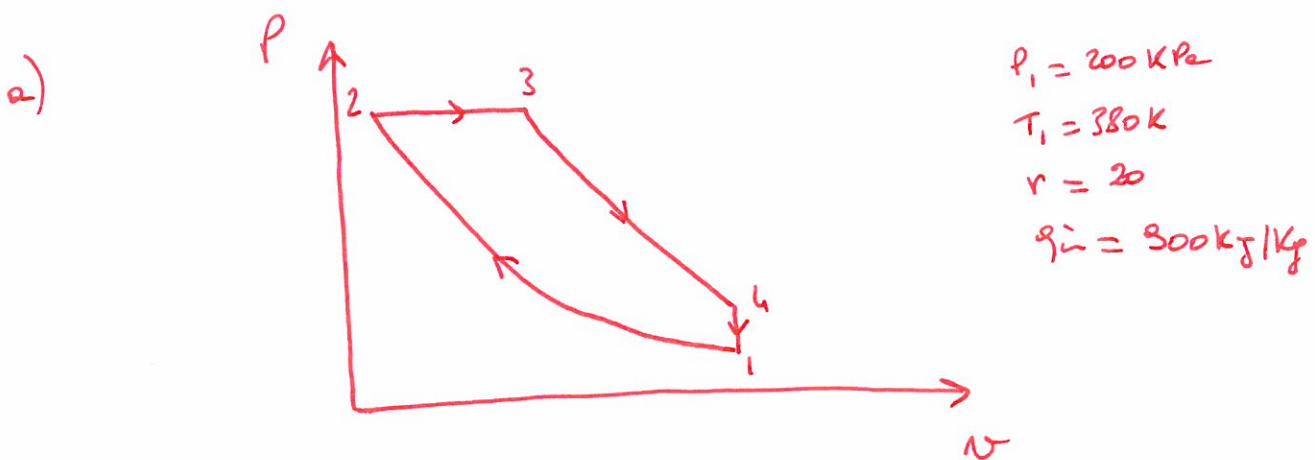
b) A-2:       $R = 0.287 \text{ kJ/kg.K}$        $c_p = 1.005 \text{ kJ/kg.K}$
